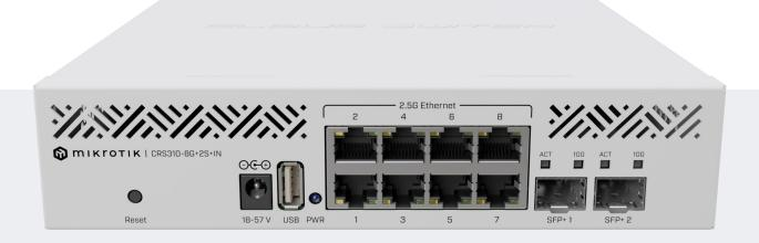
The amazing Marvell 98DX226S switch-chip and integrated dual-core ARM CPU can handle the full potential of RouterOS v7. Run VLANs, Jumbo frames, link aggregation, ACL rules, and so much more! You can even do some hardware offloaded Layer-3 routing.
